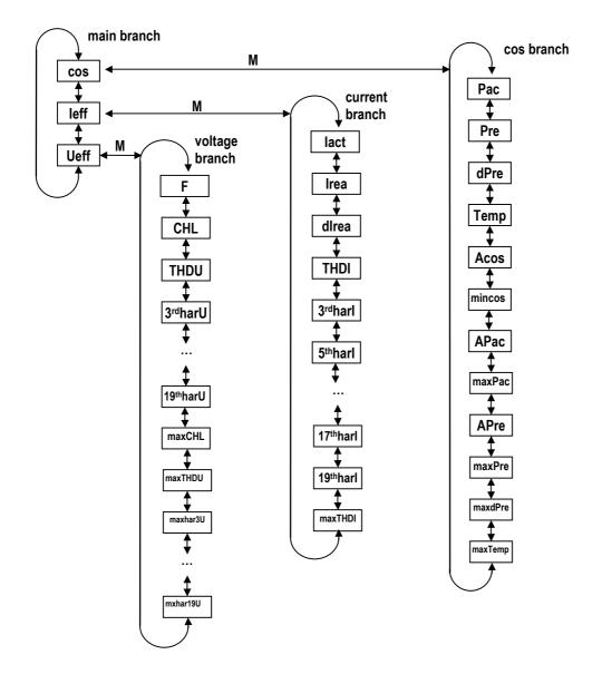
Figure 1.2: Instantaneous value display – structure
