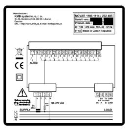
Maximum cross section area of connection wires is 2.5 square millimetres.
