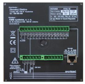
Fig. 2.6 : Controller with Ethernet Interface Rear Panel
