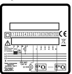
Fig. 5.3 : Novar-1005T – connector
